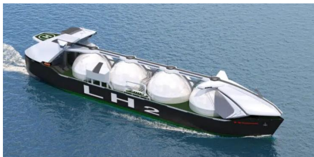
Figure 11. Kawasaki Heavy Industries – CG prototype for a commercial sized liquefied hydrogen carrier [28]
